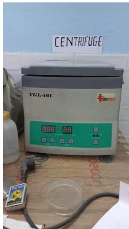
A **centrifuge** is a device that uses centrifugal force to subject a specimen to a specified constant force, for example to separate various components of a fluid. This is achieved by spinning the fluid at high speed within a container, thereby separating fluids of different densities (e.g. cream from milk) or liquids from solids.
