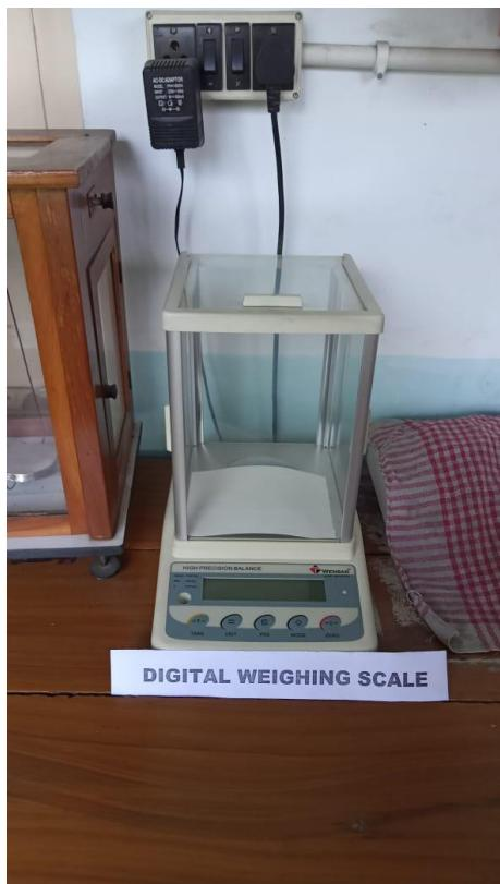
**Digital weighing scales** are devices used to measure the weight or mass of an object. They are sometimes called electronic scales and are usually composed of an LCD screen, load cell, controller and platform.
