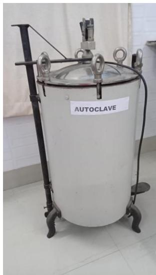
**Autoclaves** provide a physical method for **disinfection and sterilization**. They work with a combination of steam, pressure and time. Autoclaves operate at high temperature and pressure in order to kill microorganisms and spores.
